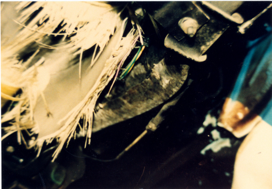
16. Closeup View of the Cylinder Flap and Frame Rail Deformation
